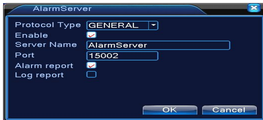
Pic: 4.30 alarm server setting
