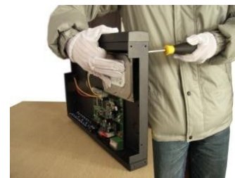
③fix the screw of hard disk
