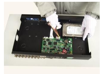
⑥connect the power wire
